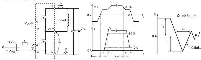
Switching characteristics test circuit and waveforms
