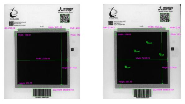
Common inspections<sup>\*</sup> in LiB applications are measurements of the anode/cathode, sort surface defects, barcode reading and grading.
